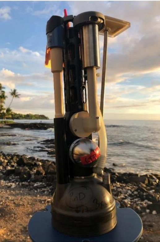
**New Seabird oxygen sensor (SBE83)** with air calibrations and faster response time from the pumped flow stream
