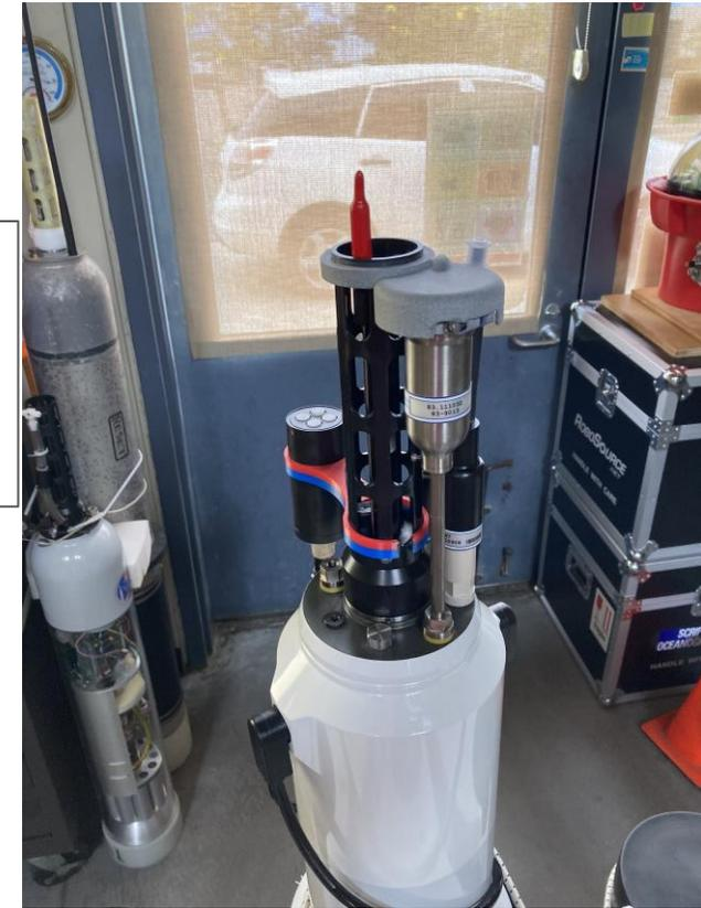
**Radiometers added to 5 (now 6) sensor Apex floats**
